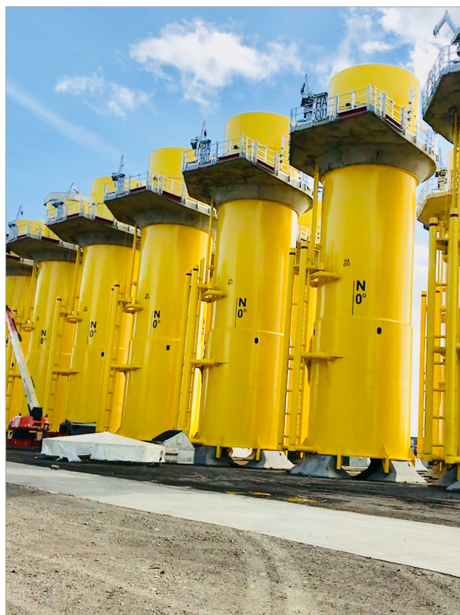
Offshore wind tower transition pieces fabricated at Wilton Engineering
