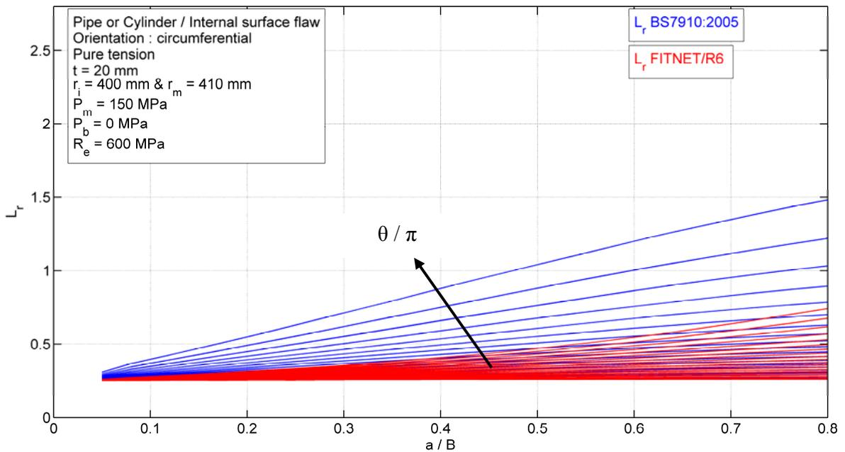
**FIGURE 31: PIPE/CYLINDER CONTAINING CIRCUMFERENTIAL INTERNAL SURFACE FLAW
