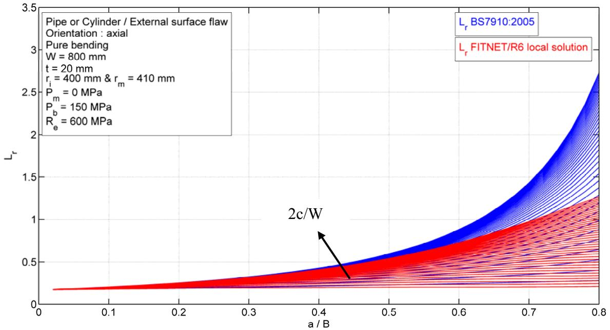
**FIGURE 22: PIPE/CYLINDER CONTAINING AXIAL EXTERNAL SURFACE FLAW
