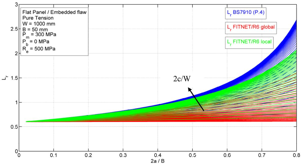
FIGURE 15: FLAT PLATE CONTAINING EMBEDDED FLAW
