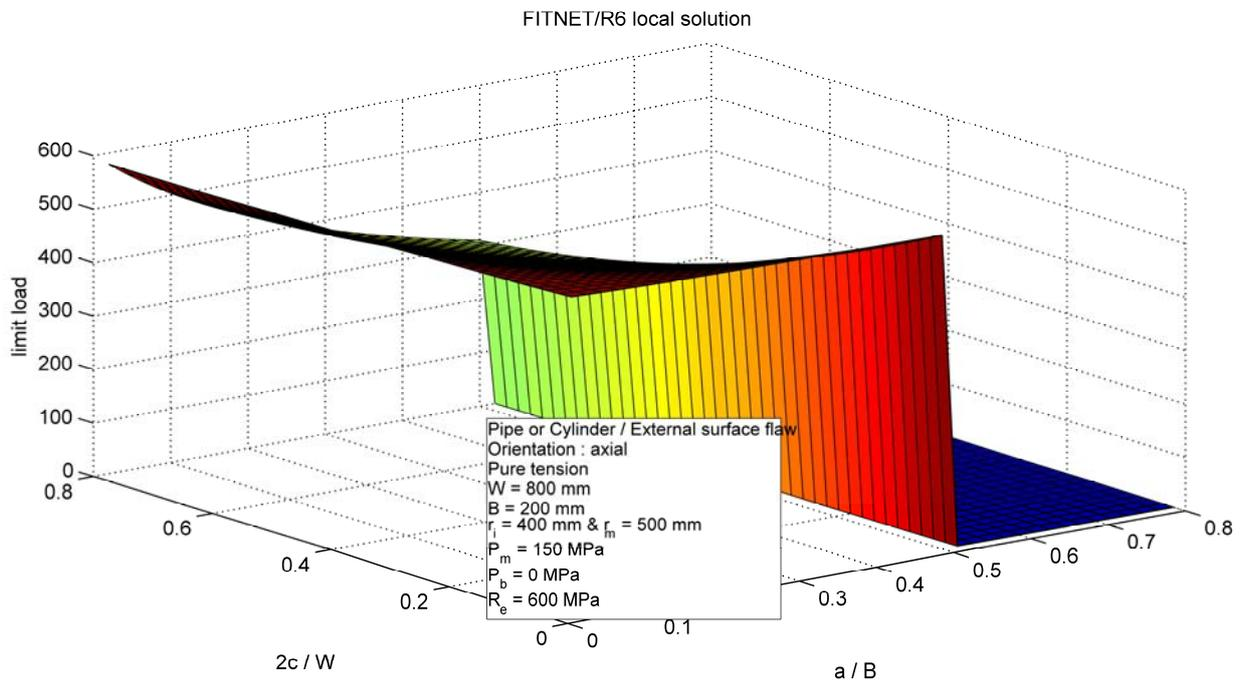
**FIGURE 25: PIPE/CYLINDER CONTAINING AXIAL EXTERNAL SURFACE FLAW
