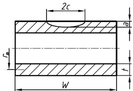
FIGURE 6: PIPE/CYLINDER WITH AXIAL EXTERNAL SURFACE FLAW [4]
