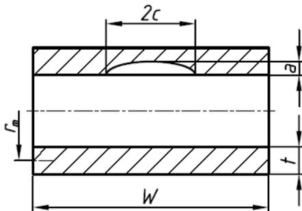
FIGURE 5: PIPE/CYLINDER WITH AXIAL INTERNAL SURFACE FLAW [4]
