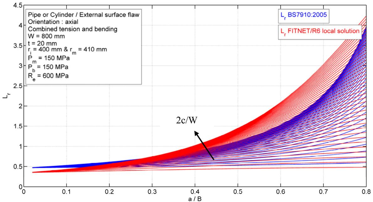
**FIGURE 23: PIPE/CYLINDER CONTAINING AXIAL EXTERNAL SURFACE FLAW
