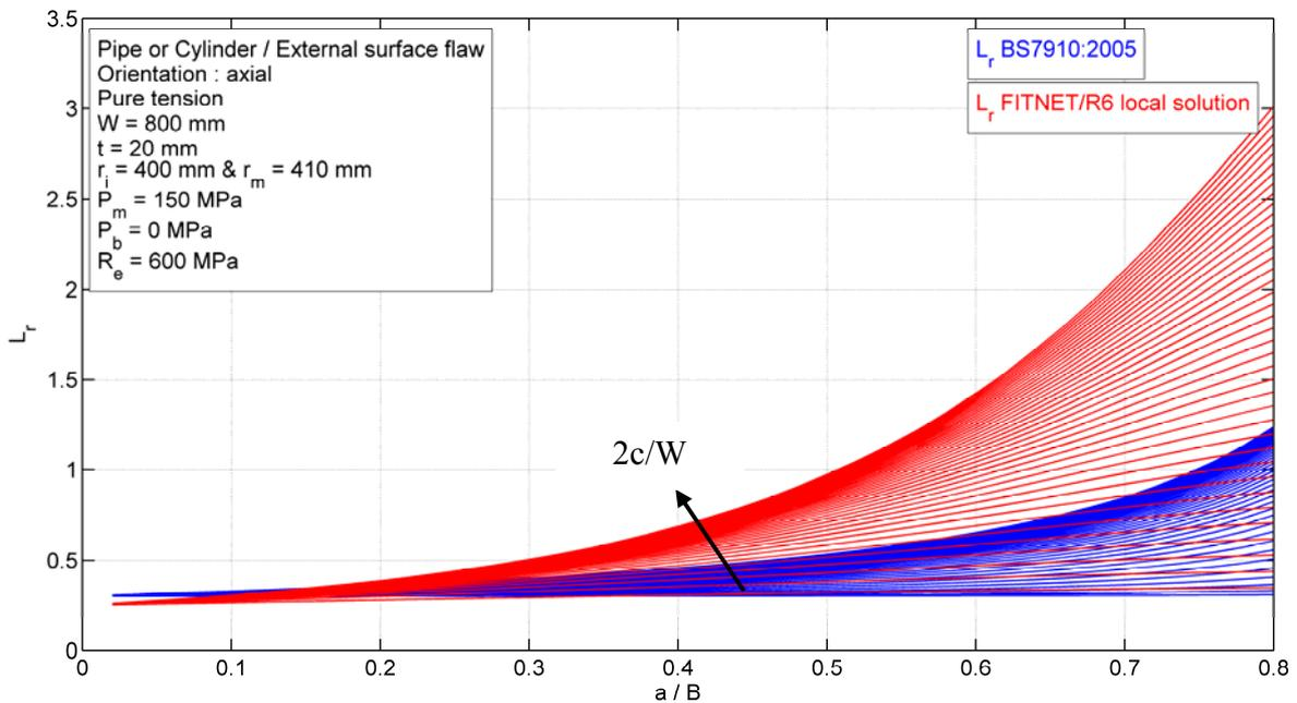
**FIGURE 21: PIPE/CYLINDER CONTAINING AXIAL EXTERNAL SURFACE FLAW
