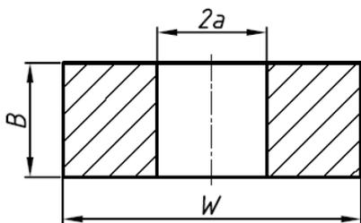
**FIGURE 1: CROSS-SECTION OF A FLAT PANEL WITH THROUGH-THICKNESS FLAW [4]**
