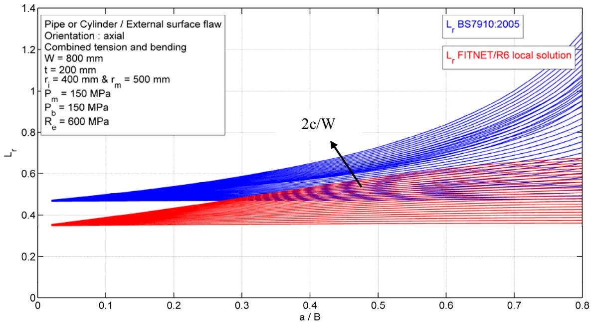
**FIGURE 27: PIPE/CYLINDER CONTAINING AXIAL EXTERNAL SURFACE FLAW
