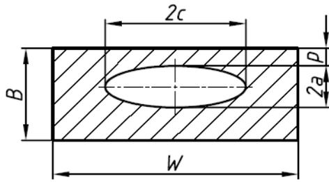
FIGURE 3: CROSS-SECTION OF A FLAT PANEL WITH EMBEDDED FLAW [4]
