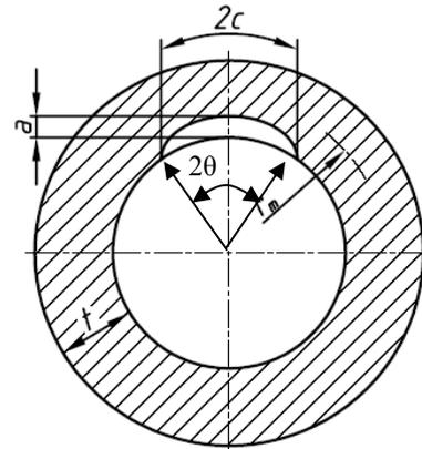
FIGURE 8: PIPE/CYLINDER WITH CIRCUMFERENTIAL INTERNAL SURFACE FLAW [4]
