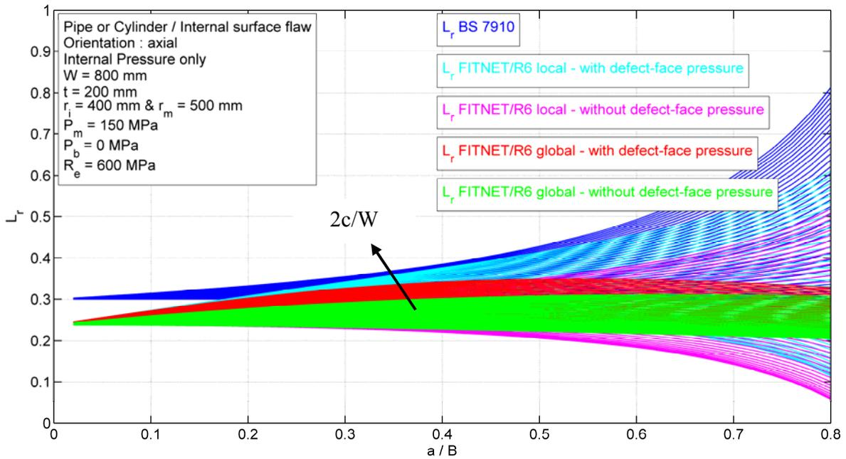
**FIGURE 20: PIPE/CYLINDER CONTAINING AXIAL INTERNAL SURFACE FLAW
