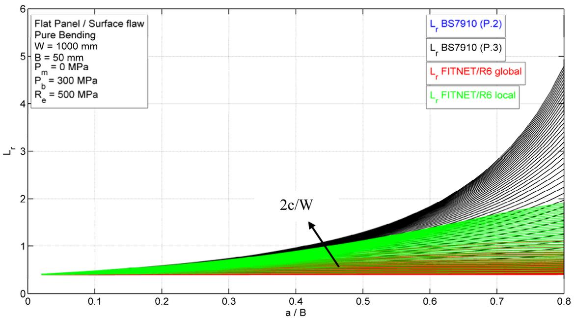
FIGURE 13: FLAT PLATE CONTAINING SURFACE FLAW
