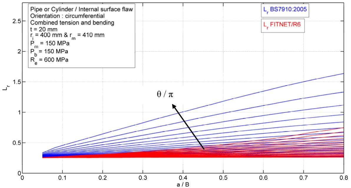
**FIGURE 32: PIPE/CYLINDER CONTAINING CIRCUMFERENTIAL INTERNAL SURFACE FLAW
