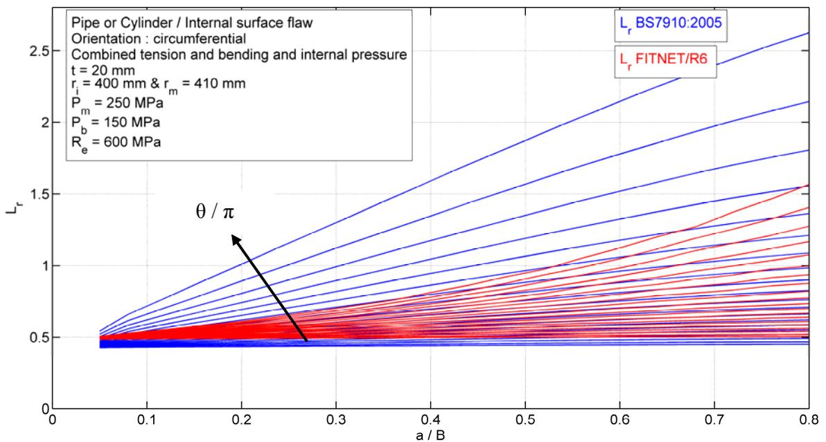
**FIGURE 33: PIPE/CYLINDER CONTAINING CIRCUMFERENTIAL INTERNAL SURFACE FLAW
