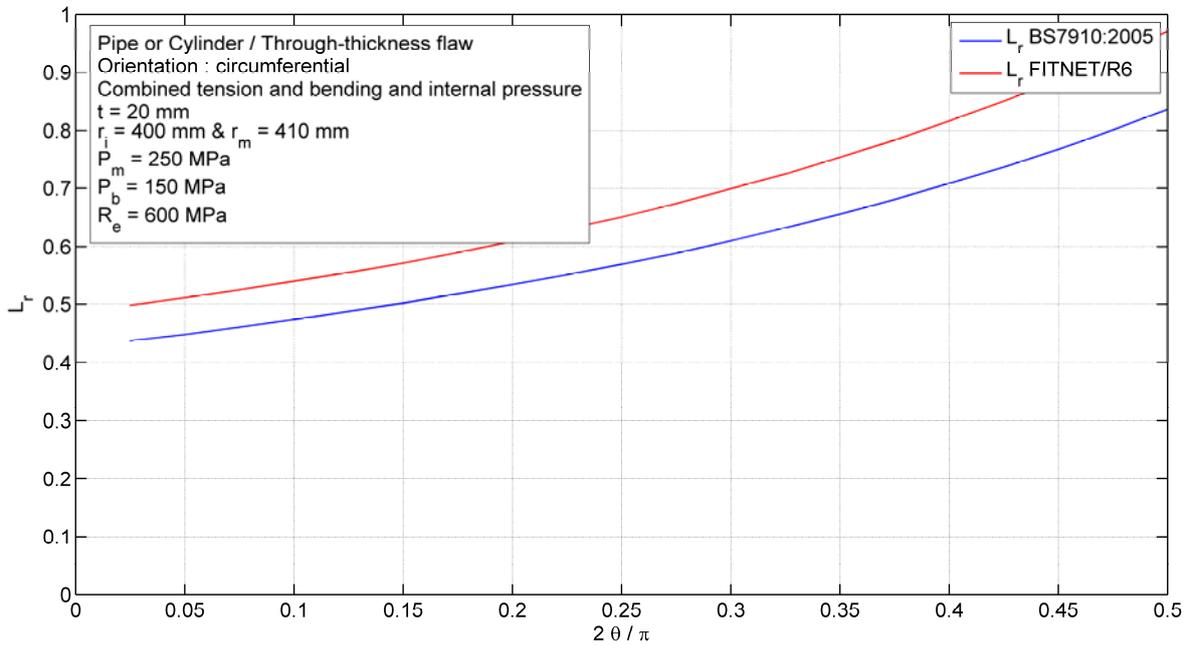
**FIGURE 30: PIPE/CYLINDER CONTAINING CIRCUMFERENTIAL THROUGH-THICKNESS FLAW
