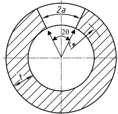
FIGURE 7: PIPE/CYLINDER WITH CIRCUMFERENTIAL THROUGH-THICKNESS FLAW [4]
