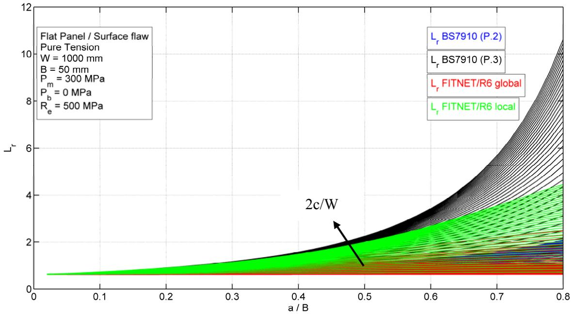
FIGURE 12: FLAT PLATE CONTAINING SURFACE FLAW
