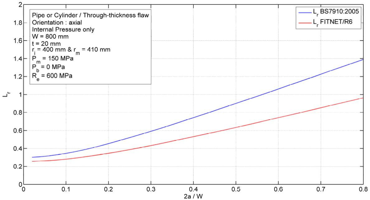
**FIGURE 18: PIPE/CYLINDER CONTAINING AXIAL THROUGH-THICKNESS FLAW
