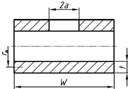
FIGURE 4: PIPE/CYLINDER WITH AXIAL THROUGH-THICKNESS FLAW [4]
