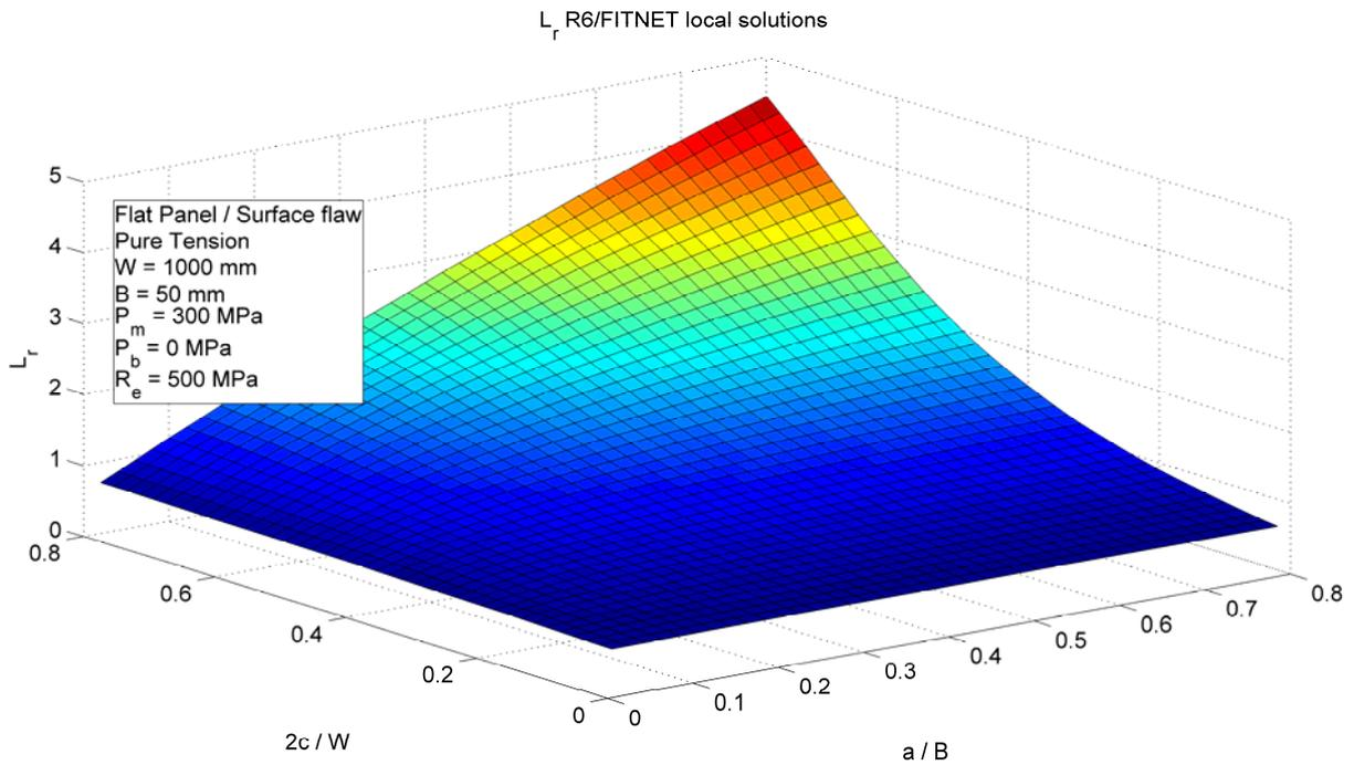
**FIGURE 11: FLAT PLATE CONTAINING SURFACE FLAW – PURE TENSION
