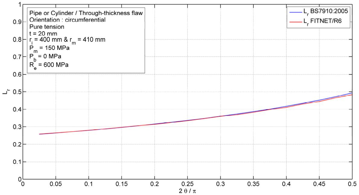
**FIGURE 28: PIPE/CYLINDER CONTAINING CIRCUMFERENTIAL THROUGH-THICKNESS FLAW
