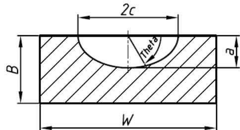
**FIGURE 2: CROSS-SECTION OF A FLAT PANEL WITH SURFACE FLAW [4]**
