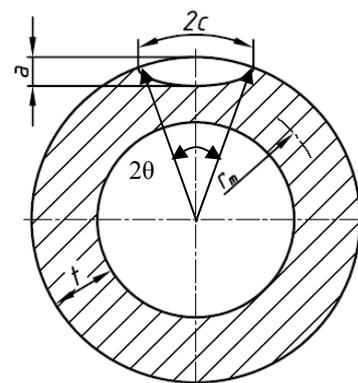
FIGURE 9: PIPE/CYLINDER WITH CIRCUMFERENTIAL EXTERNAL SURFACE FLAW [4]
