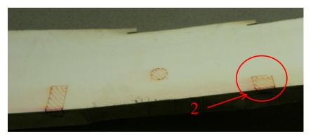
Trial on defect 2 (25mmx25mmx1mm) in foam located 5mm under gel coat
