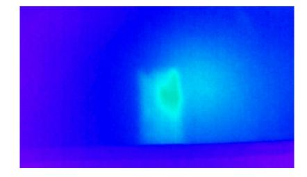
Trial on defect 1 (25mmx50mmx5mm) in GPRF located under gel coat
