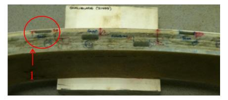
Trial on defect 1 (25mmx50mmx5mm) in GPRF located under gel coat
