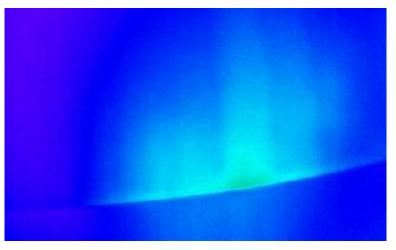
Trial on defect 2 (25mmx25mmx1mm) in foam located 5mm under gel coat
