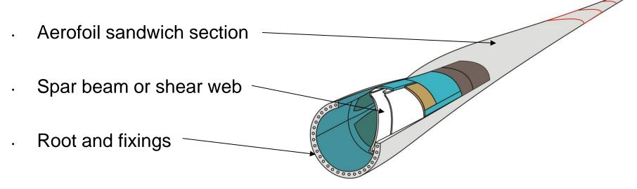
There are design and material differences between each of the manufactures blades, and inspection selection will be affected by these differences.
