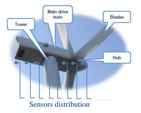
16 inputs @ 2MSam/Sec for AE SHM 16 inputs @ 250KSam/Sec for CM 16 parametric inputs
