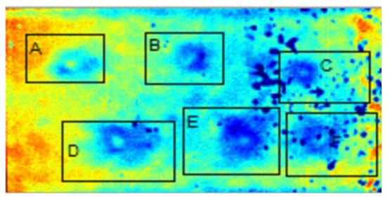
Disbonds in wind turbine blade detected by thermography
