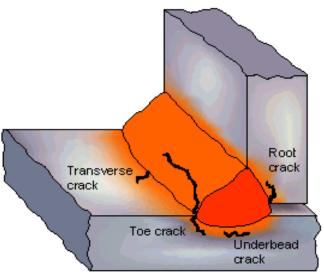
Fig. 1 Hydrogen cracks originating in the HAZ (note, the type of cracks shown would not be expected to form in the same weldment)
