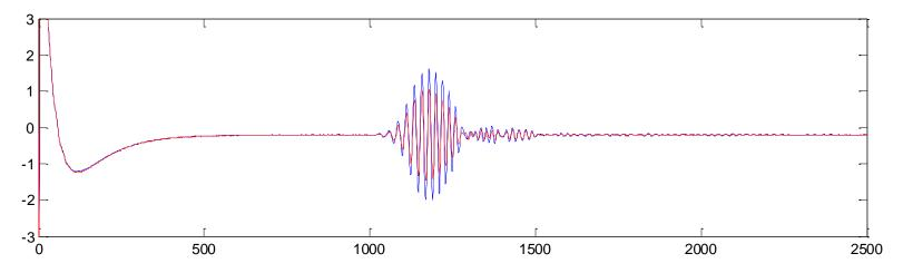
The normalize cross-correlation between different signals at longest distance (the hole on the path)
