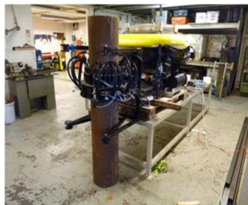
LRUT mounting on an ROV
