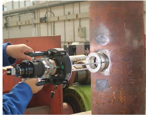
Figure 1 Rapid CreepImage inspection performed using a camera positioning jig.
