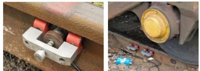
Off-the-shelf PAUT data acquisition was used, and the value added by the SAFERAIL project was in the development of the inspection techniques and unique deployment of the PAUT probes. Probe holders including encoders have been developed and together with level two written procedures offer reliable inspection solutions for both axles and wheels.
