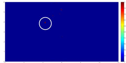
Thresholded image of the plate showing the defect detected by the ShipInspector sensor array
