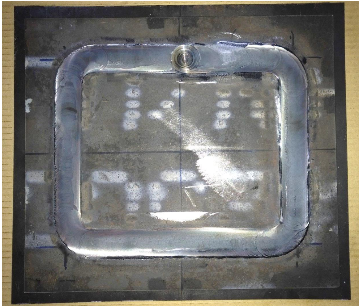
Figure 4. Image of a DH36 steel 'patch' lap welded to a 12mm thick S460 'hull' plate.
