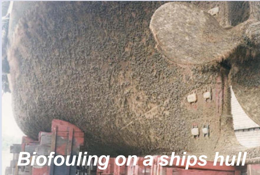
*Biofouling on a ships hull*
