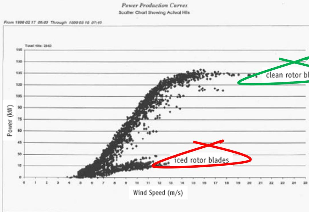
Fouling can cause significant loss of efficiency
