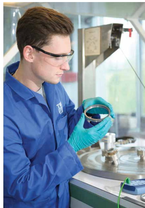
Alex Russell inspecting a joint made using diffusion bonding and brazing with the aid of interlayers, for the European Space Agency
