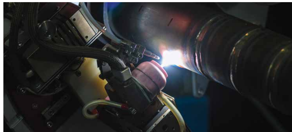
Welding trials on thin-wall duplex steel pipe
