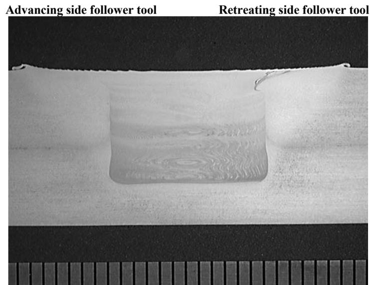
**Fig 8.** Macrosection of Tandem Twin-stir™ lap weld in 6 mm thick 6082-T6 aluminium alloy
