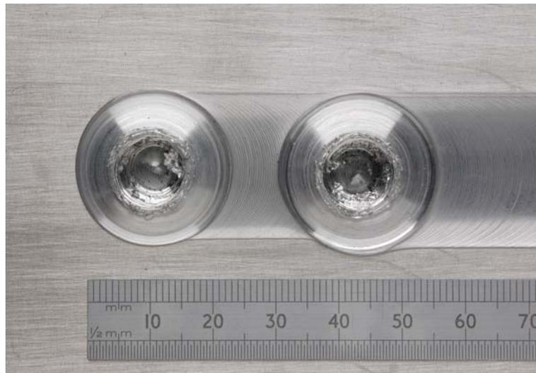
**Fig 7.** Tandem Twin-stir™ lead and follow exit holes
