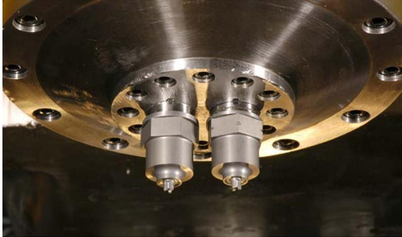
**Fig 5.** Twin-stir™ prototype head assembly
