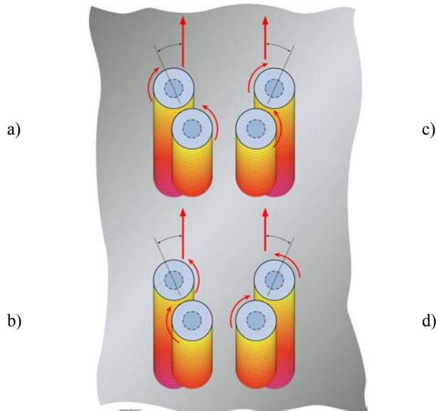
**Fig 4.** Arrangement of Staggered Twin-stir™ contra-rotating tools with respect to rotation and direction
