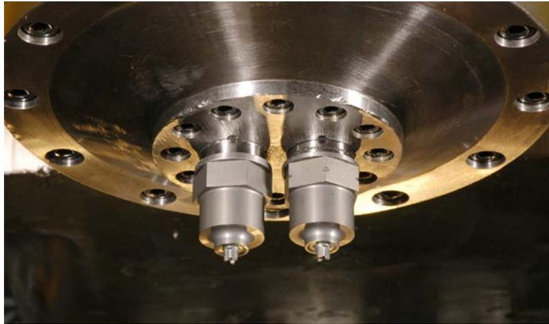
**Fig 5.** Twin-stir™ prototype head assembly
