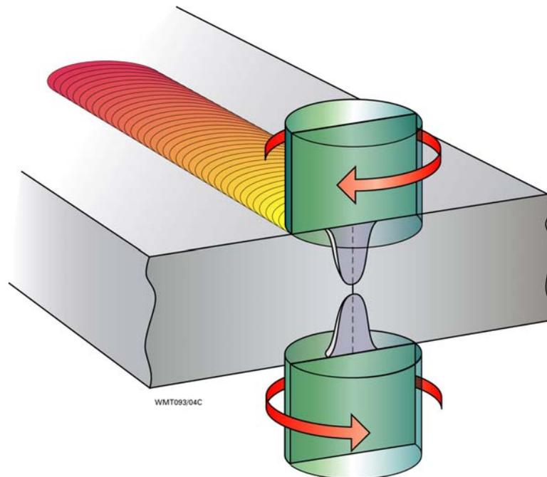
**Fig 1.** Simultaneous double-sided friction stir welding with contra-rotating tools.
