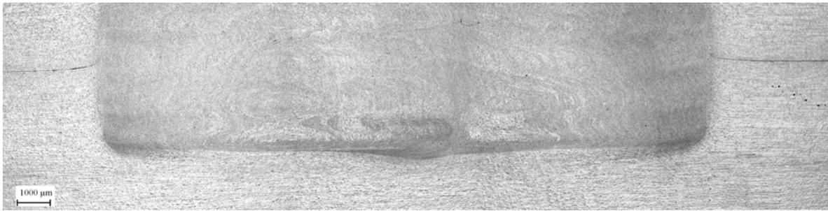
**Fig 9.** Montage of macrosections taken from the ‘common weld region’ of a Staggered Twin-stir™ weld
