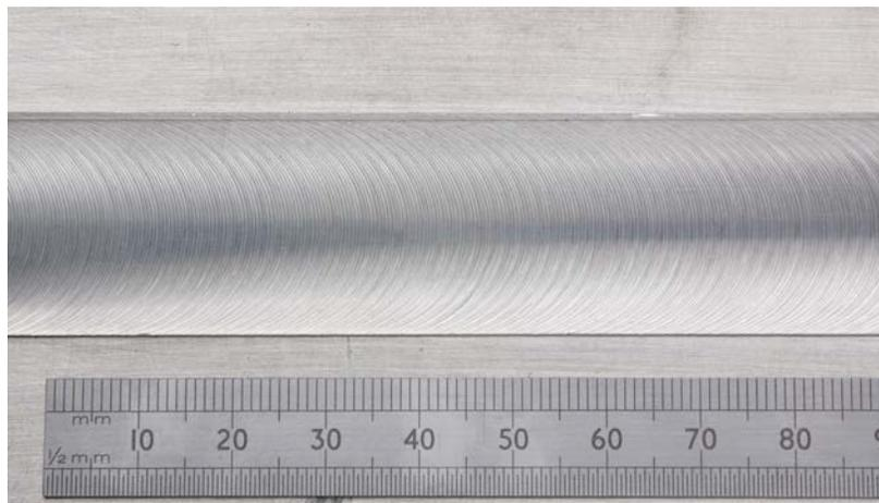
**Fig 6.** Surface appearance of a typical Tandem Twin-stir™ weld made in 6083-T6 aluminium alloy
