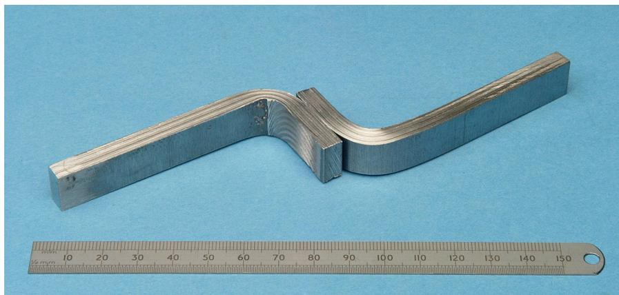
**Fig. 7 Hammer ‘S’ bend of a Re-stir™ lap weld made in 5083-O condition aluminium alloy material showing good weld integrity**
