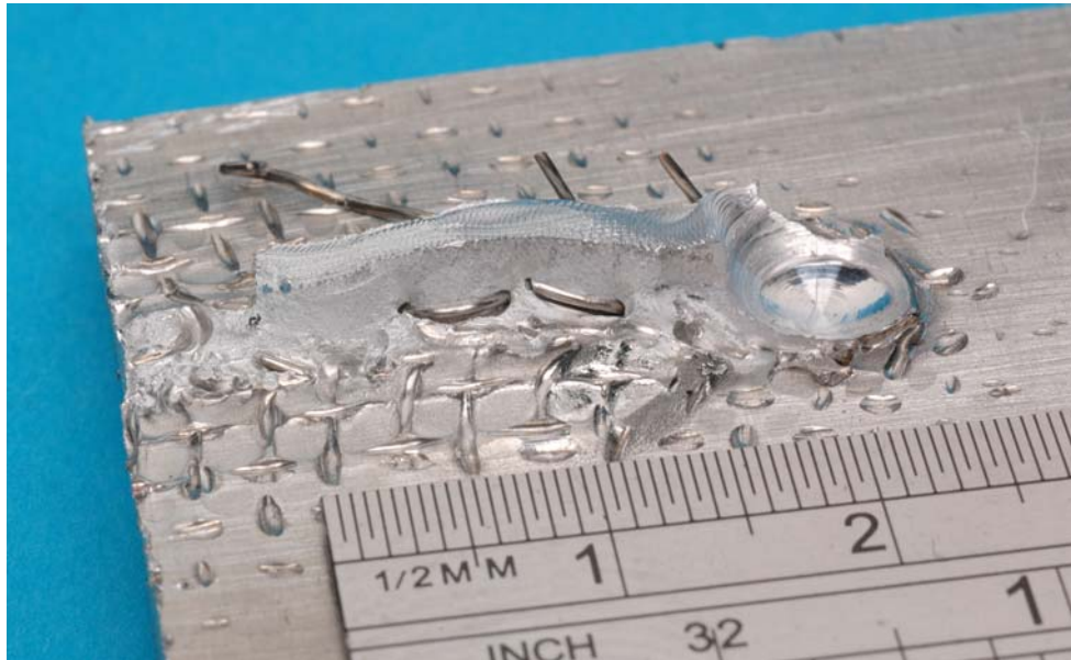
Fig. 5 Transition joint between stainless steel mesh and aluminium sheets
