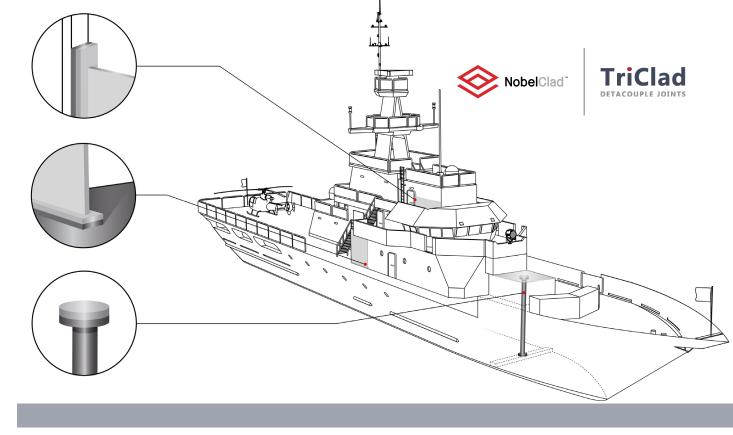
TriClad® aluminium-steel transition joints are used to provide an efficient and maintenance free welded connection between aluminium and steel structures on board vessels.
