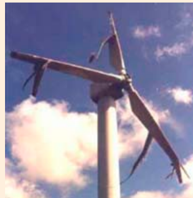
Damaged wind turbine blades
