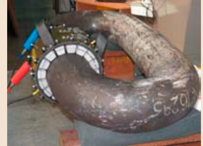
Inspection of chain link
