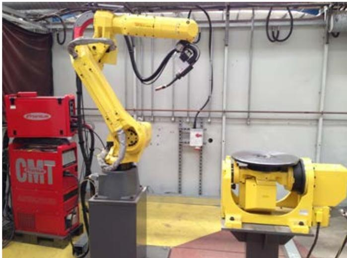
Figure 1. Robotic AM system at TWI
