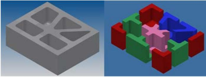
Figure 2. Relatively simple AM part made from ten separate sub-shapes
