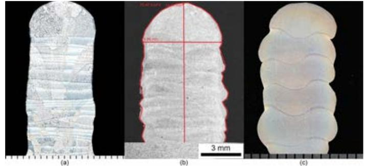
Figure 3 shows macro sections of Ti-6Al-4V, AA 4043 and IN718 arc-based AM walls
