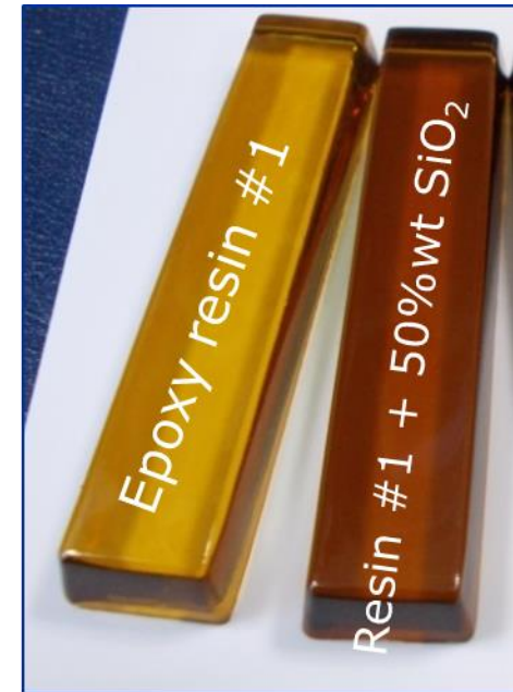
Figure 2 Epoxy resin blocks with and without ~50%wt of silica loading
