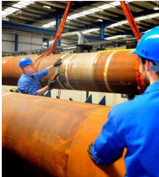
Rust develops on steel during transportation, handling and storage. → Material waste and higher costs
