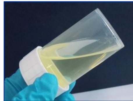
Figure 1 Low viscosity epoxy resin with ~50%wt in silica nanoparticles loading
