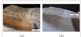
Weld cap HAZ obtained with: (a) Rutile electrodes; (b) Oxyrutile electrodes.
