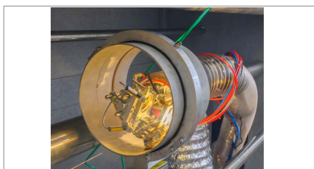
The snake arm integrated, multi-positional in-bore laser system, in operation in TWI's laboratory.
