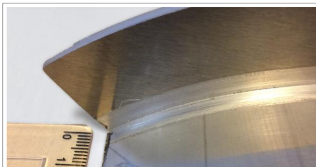
Corner SSFSW of a rib onto a curved aluminium sheet
