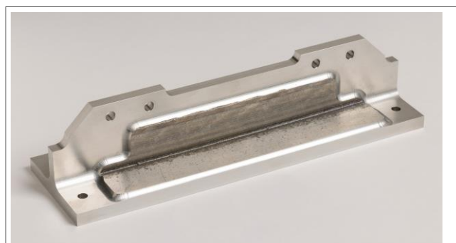
Photograph of the wing rib post demonstrator showing a region of the original deposit surface
