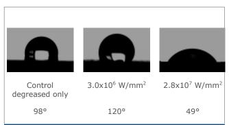
Contact angle measurements: water droplets on PP treated at different laser intensities
