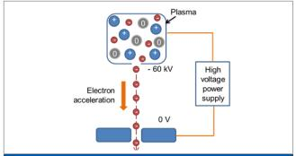
Diagram showing an electron beam extracted from a plasma
