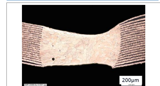
Single-pass 20 lap-welded copper foils, each of 17 \mu m thickness (electrical connection applications).
