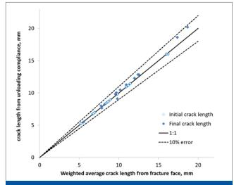
Validation of crack lengths estimated from unloading compliance against measurements from fracture faces
