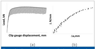
The unloading compliance method, uses the slope from partial unloadings during the test (a), to estimate crack extension,  $\Delta a$ , to plot R-curves (b).
