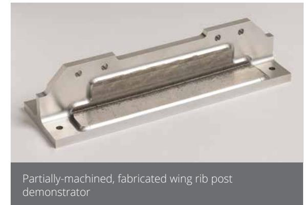
Partially-machined, fabricated wing rib post demonstrator
