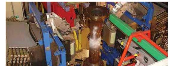
Measurement of residual strains in the axially strained pipe spool
