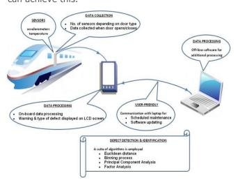
The proposed system for remote condition monitoring using vibration analysis (VA-RCM) for train door control systems will automatically detect wear in door rollers, the linear shaft assembly, ball bearings and misalignments in the shaft and door panels in the very early stages, before breakdown of the door mechanisms occur. Early stage fault
