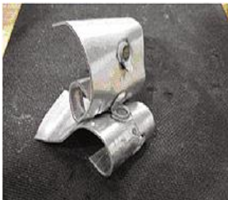
The destructive peel test
