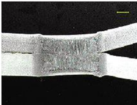
Cross section of a basic spot weld
