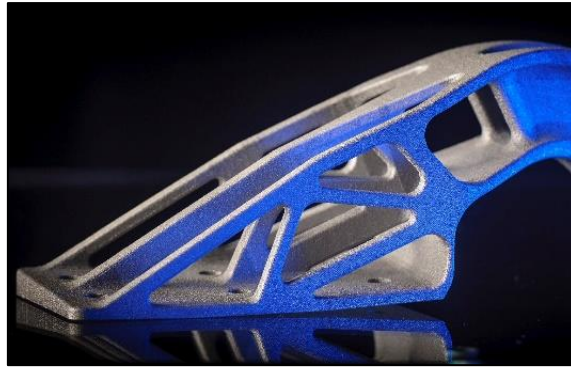
Figure 3 LB-PBF component manufactured at TWI Ltd ( Courtesy of TWI Ltd. )
