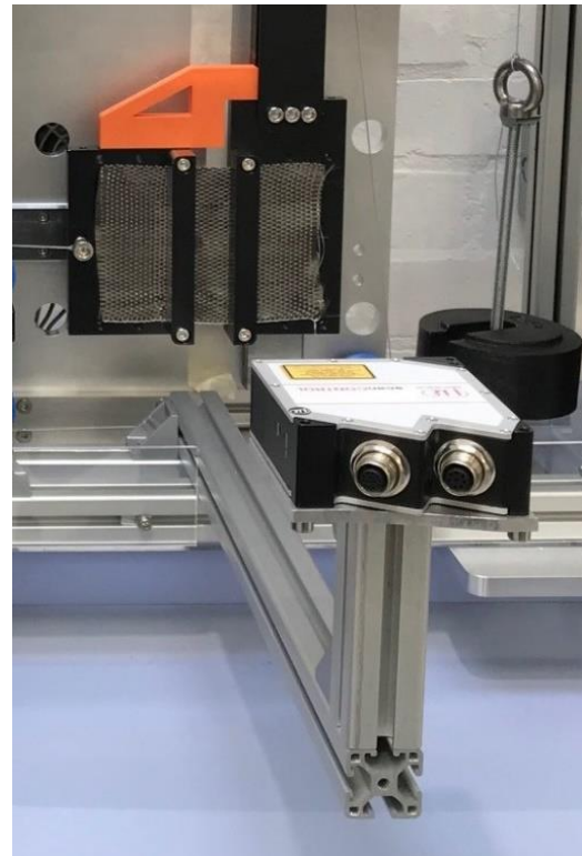
Figure 2: Shear rig developed by iCOMAT for the assessment of material characteristics for iCOMAT's process, i.e. shear rate, maximum shear angle etc.
