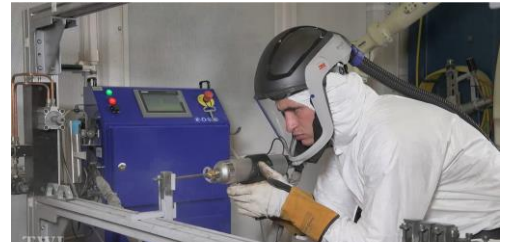
Example of manual, low pressure cold spray being performed.
