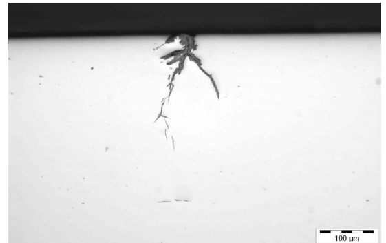
Sour stress corrosion cracking in wrought 316L austenitic stainless steel
