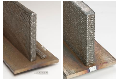
Typical AM test specimens made by arc welding using wire consumables
