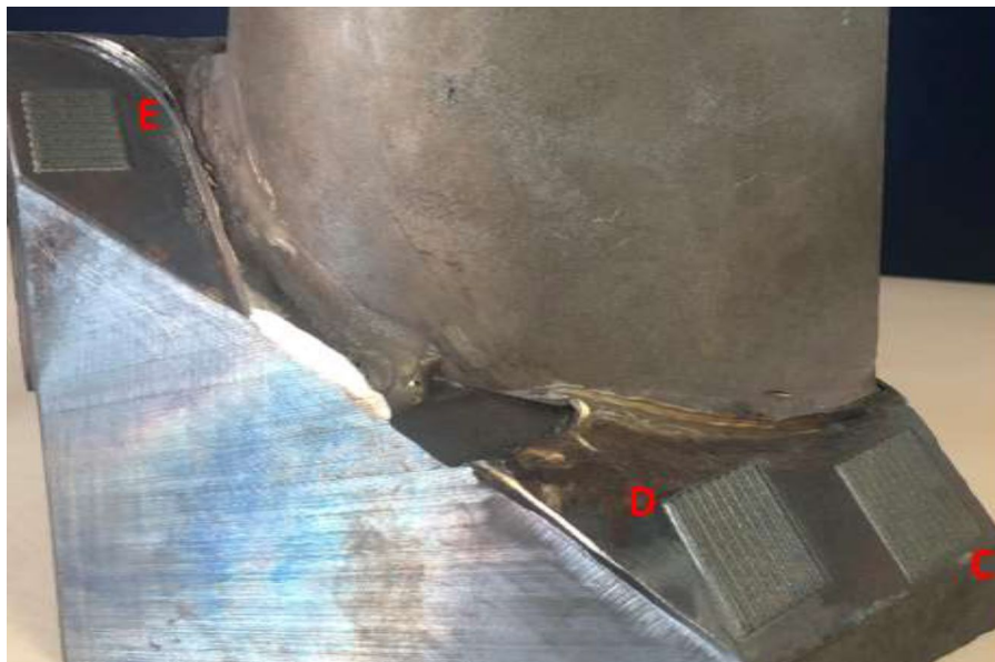
Figure 1 - Turbine component for testing at ON with three coating areas
