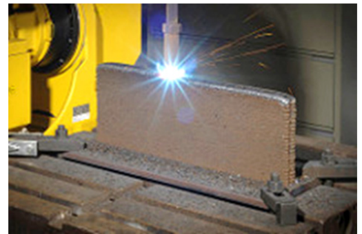
Arc and Wire AM parts can exhibit unusual microstructures, the effect of these on joining processes needs further investigation
