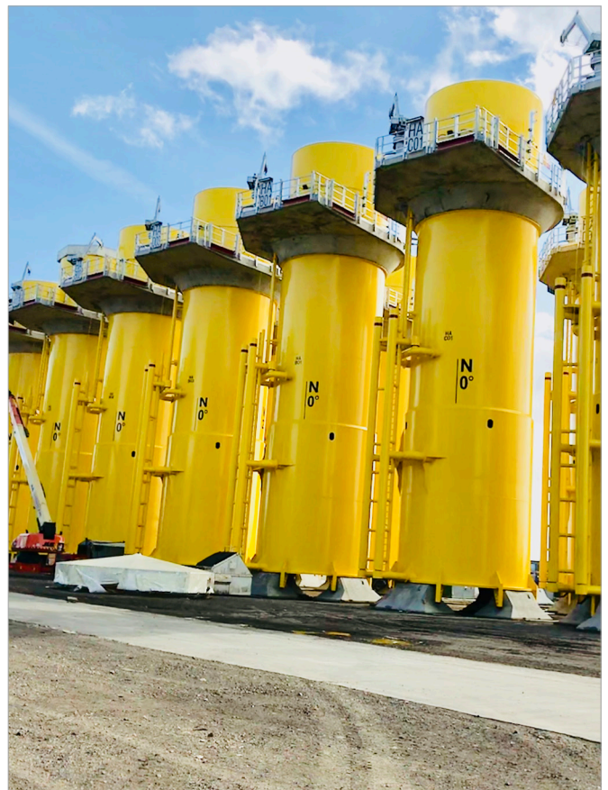
Offshore wind tower transition pieces fabricated at Wilton Engineering
