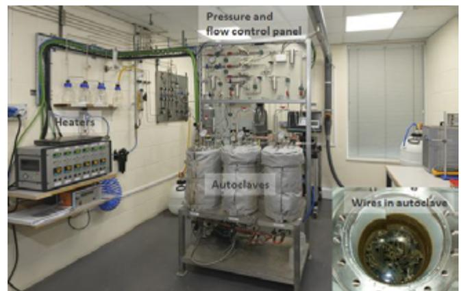
**Figure 2.** Laboratory for simulated annulus testing.
