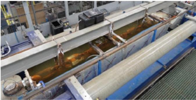
**Figure 1** Full-scale fatigue test set-up in free corrosion conditions in seawater.
