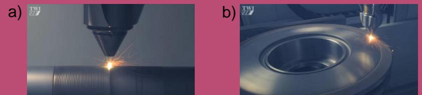
Figure 3: a) The EHLA process coating a hydraulic cylinder (TWI, n.d.) b) EHLA coated brake discs (TWI, n.d.)
