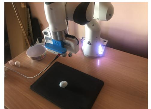
Figure: Real-World evaluation setup based on the Franka Panda Robot an Intel Real-Sense D455 RGB-D camera & 3D printed mushrooms.
