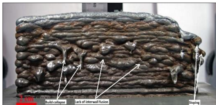
Example of sloping & Build collapse in a maraging steel 4
