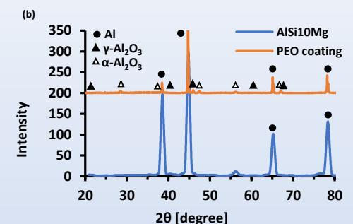
Figure 6: SEM of PEO coating surface and XRD analysis of As-built and coated configuration
