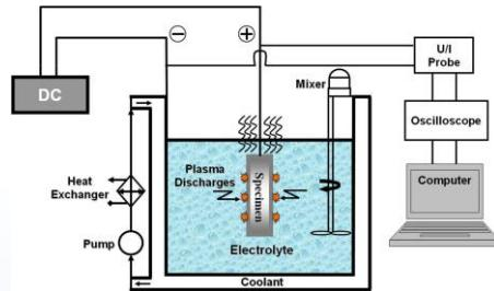
Figure 1: Functional diagram for the Plasma Electrolytic Oxidation (PEO) system [1].
