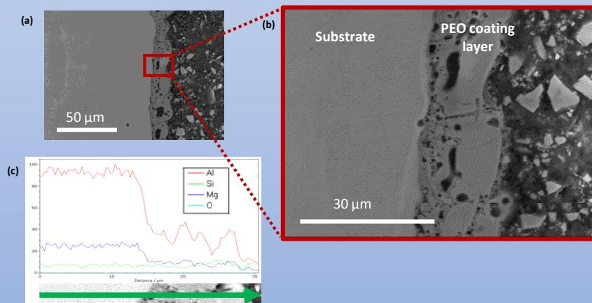
Figure 3: (a) SEM micrograph of PEO layer; (b) detail at higher magnification of the coating layer; (c) EDX analysis for thickness valuation
