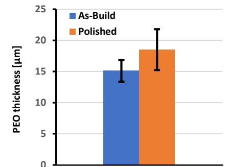
Figure 4: PEO Layer thickness measurement for the two configuration (polished and not polished)
