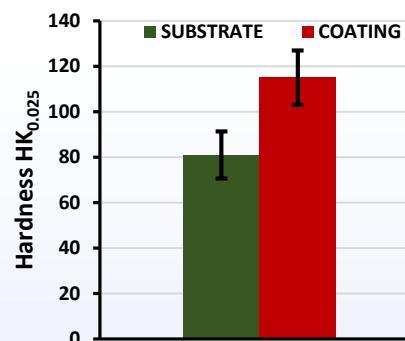
Figure 5: Microhardness of substrate and PEO coated layer
