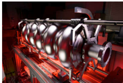
EB welded niobium RF cavity for US mega-science project 'DUNE PIP-II' (courtesy of Fermilab USA).
