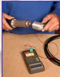
7. Check alignment of parts, clamp or tack as required.
