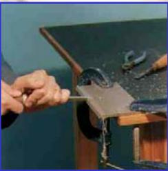
4. Apply suitable prep to weld area, typically 90° inclusive for butt weld with single-V  $\leq$  6mm thick sheet and double-V  $>$  7mm thick sheet. Apply suitable prep to pipes, considering pipe configuration, to enable root penetration.
