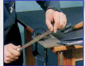
5. Scrape area to be welded, creating a smooth surface, removing just enough for the weld to cover. Do not over-scrape.
